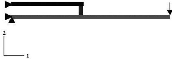
**Figure 2:** Simple FEA beam model of capacitor mounted on printed wiring board
