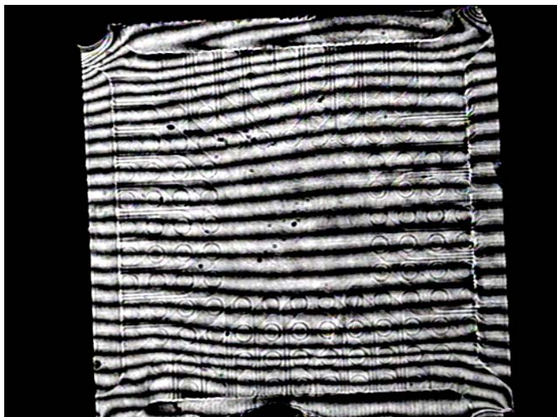
Figure 7. Moire' fringe pattern of an assembled 12 mm E-CSP. Method revealed a package CTE of 15.5 ppm/°C in the x-y direction
