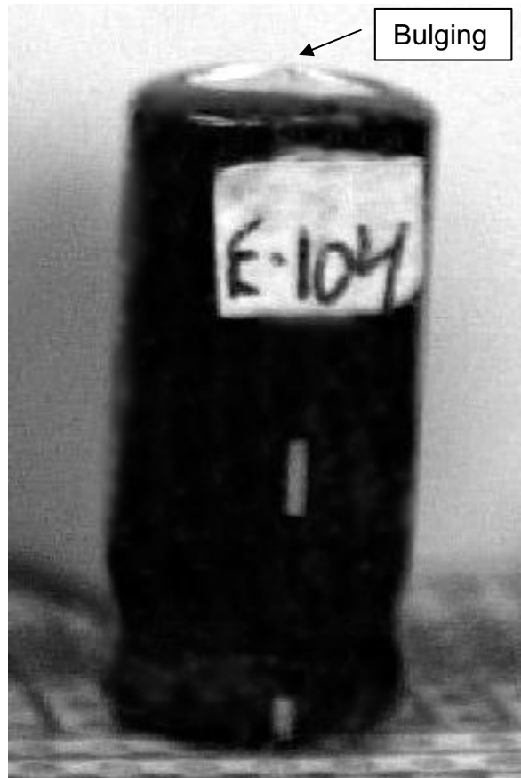
Figure 1: A bulged 1000 microfarad, 10 volt, aluminum electrolytic capacitor manufactured in Taiwan in 2002. The photograph has been retouched to obliterate manufacturer identity information.
