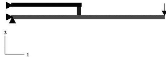
Figure 4: FEA beam model of 0805 capacitor
