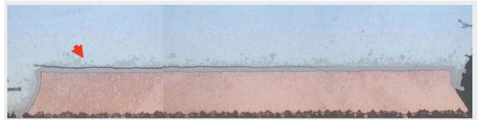
Figure 8. A brittle crack at the Ni/IMC interface in a Pb-free solder joint. This was an as-assembled board after random cross section.
