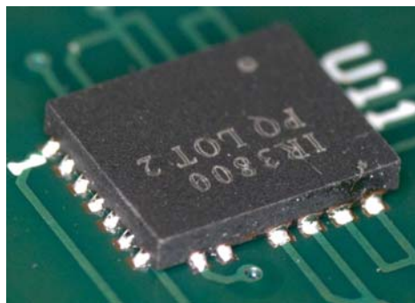
Figure: Extension of solder joints due to bond pad design
