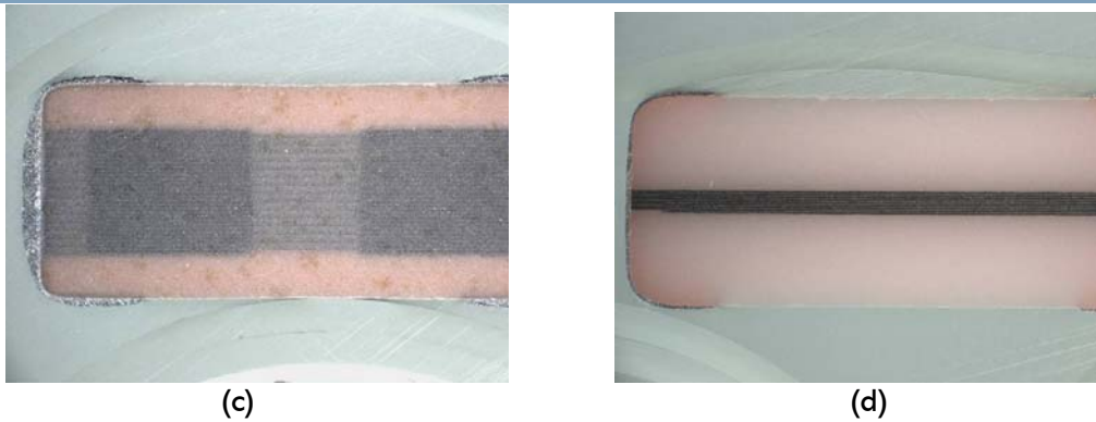
Figure 5: (a) Original Novacap capacitor, (b) Suspect capacitor, (c) Cross Section of Novacap capacitor and (d) Cross section of suspect capacitor Assessing the risk and impact of counterfeits
