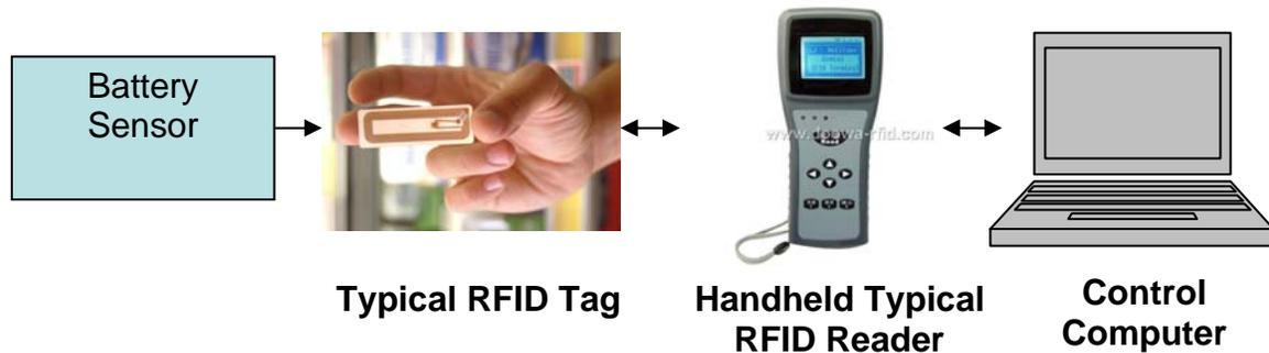
**Figure 2 – Proposed concept for Battery Sensor/RFID Measurement Approach**
