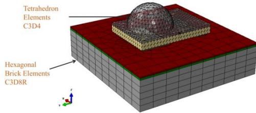
Figure 1 – Example of meshed model developed for LUXEON Rebel LED on a MCPCB
