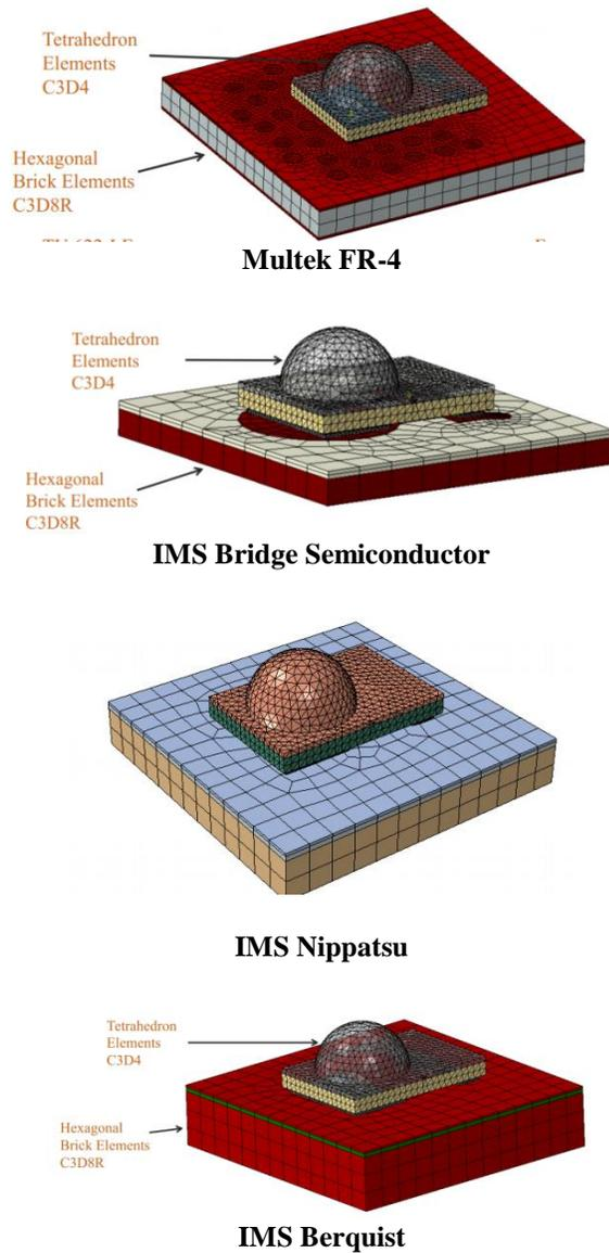
Figure 5 – Different Meshed Models
