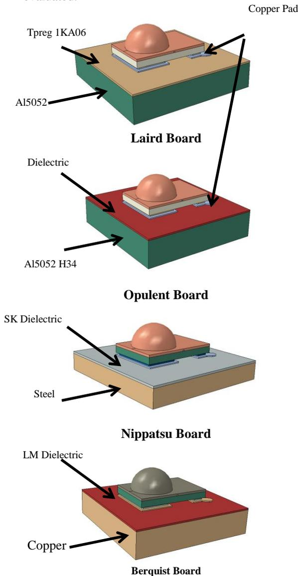
Figure 3 – Board Configurations
