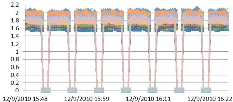
**Current draw for 32 fans after accelerated testing**
