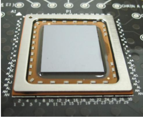
Figure 2: Coreless BGA studied
