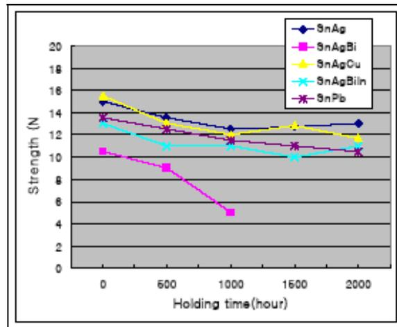
Figure 2: **Change in fracture strength after aging as a function of solder composition and SnPb plating<sup>3</sup>**
