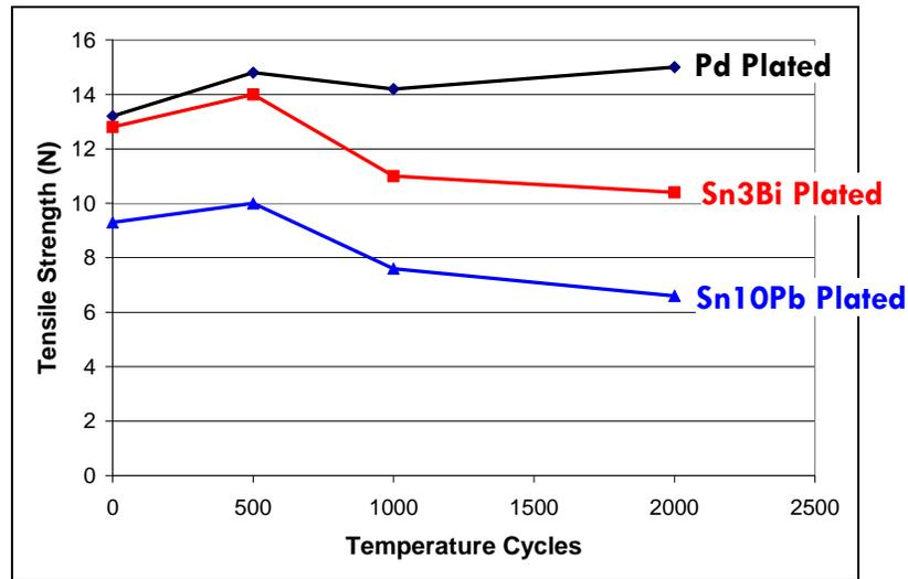
Figure 3: Tensile strength of quad flat pack (QFP) leads attached with Sn2.5Ag1.0Bi0.5Cu solder<sup>4</sup>
