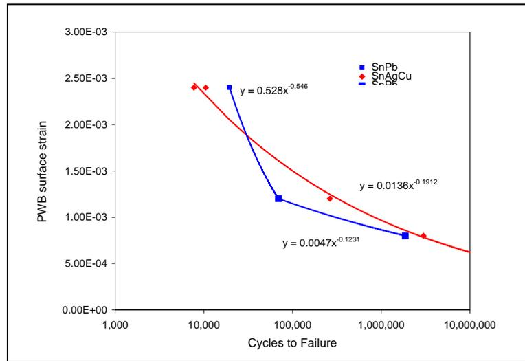
Figure 5: Cycles to failure under mechanical cycling for SnPb and SAC solder
