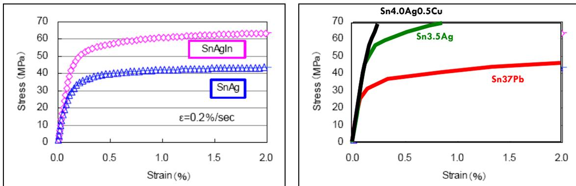
Figure 1: Stress-strain behavior of Sn-based alloys<sup>1</sup>.
