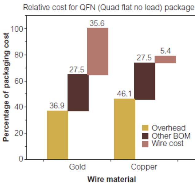
Figure 3. Comparative cost of assembling an 85 lead QFN package with gold and copper wires.<sup>1</sup>
