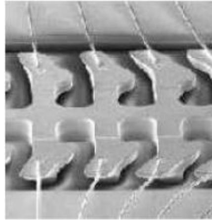
**Figure 7.** Bonding to a QFN lead can be difficult with copper, since the leads are not well supported.<sup>5</sup>
