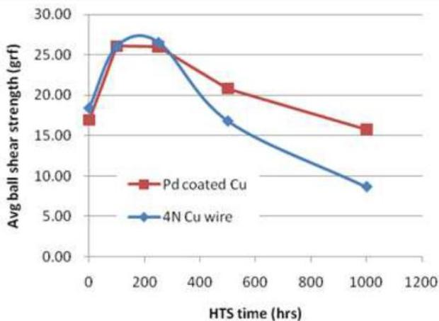
**Figure 12.** Shear strength of ball bonds after aging at  $200^{\circ}\text{C}$ .
