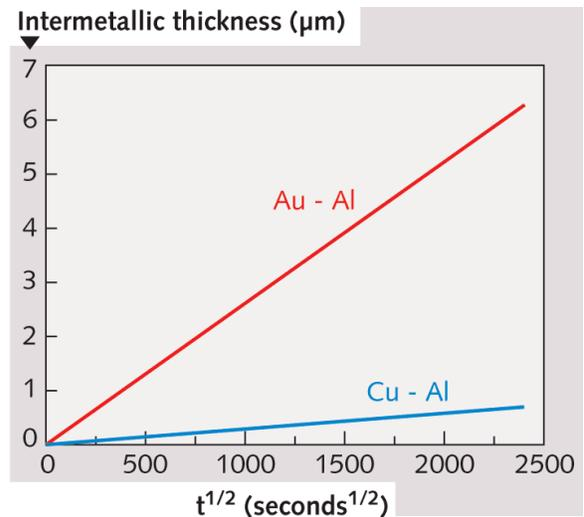
**Figure 9.** Growth of intermetallic thickness vs. time at 175°C.<sup>10</sup>
