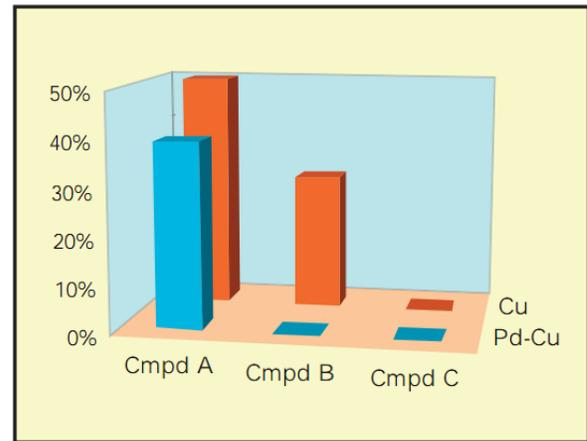
**Figure 15.** Failure rates after 336 hours biased HAST test for three mold compound formulations with 0.8 mil Cu wire on Al pads (5V bias, 130°C, 85% RH).<sup>15</sup>
