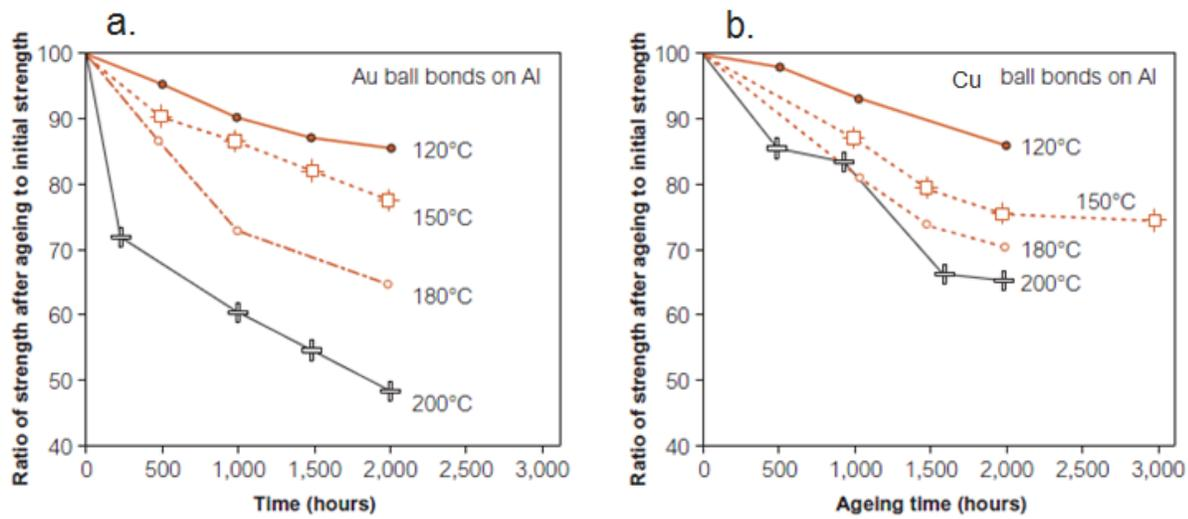
**Figure 11.** Shear strength of Au and Cu ball bonds on Al bond pads after aging. At temperatures of  $<120^{\circ}\text{C}$  they are similar after 2000 hours.<sup>9</sup>
