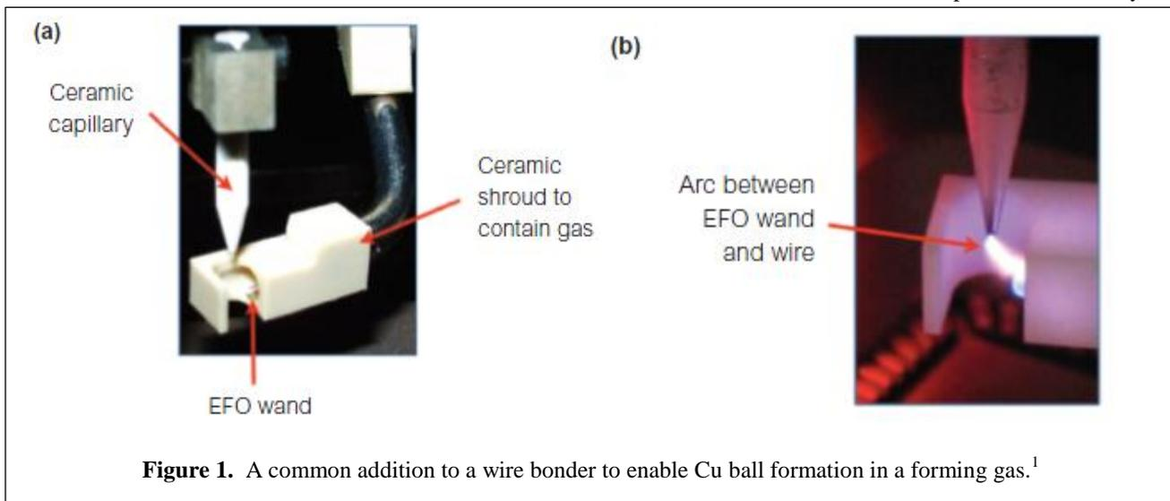
**Figure 1.** A common addition to a wire bonder to enable Cu ball formation in a forming gas.<sup>1</sup>
