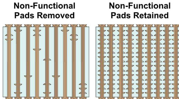
Figure 4 NFP Schematic [4]
