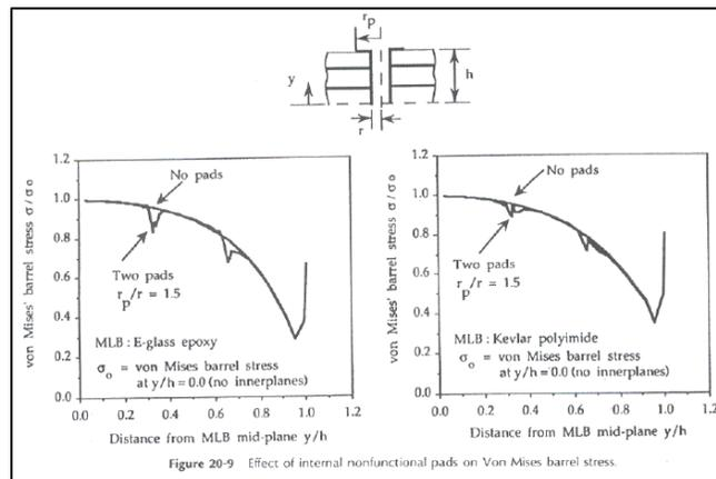
**Figure 6.** Effect of NFPs on Barrel Stress
