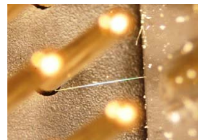
Tin whisker growing from a bright tin coated connector shell
