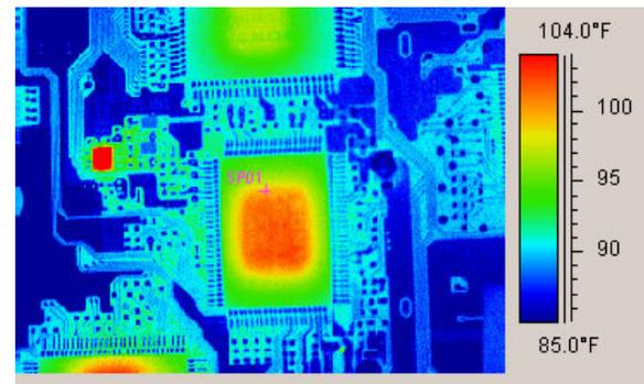
**Figure 9 – Infrared Thermography**
