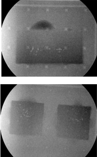
**Figure 8 – Good Diode (top image) 280V breakdown voltage; Counterfeit Diode (bottom image) 50V breakdown voltage**
