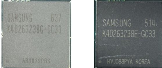
Figure 3 – Marking Registration Differences
