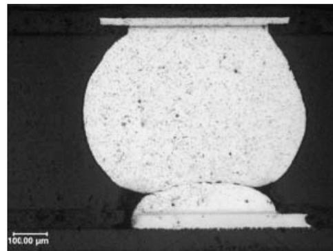
Figure 5 – Lead Free Ball on Sn/Pb Pad
