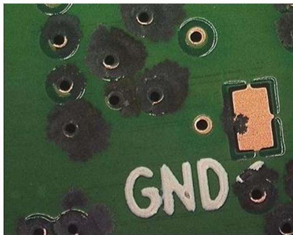
**Figure 4: Corroded Cu with OSP finish**
