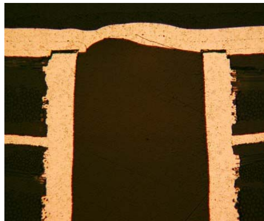
Figure 2 : Example of cap separation, no wrap plating
