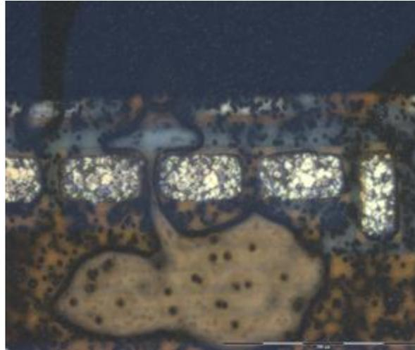
Figure 4. Large air bubble in an Chip-on-Glass ACF interconnection.
