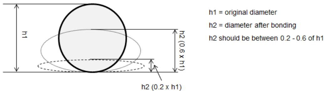
Figure 3 Recommended degree of compression for a conductive particle to ensure compliance.
