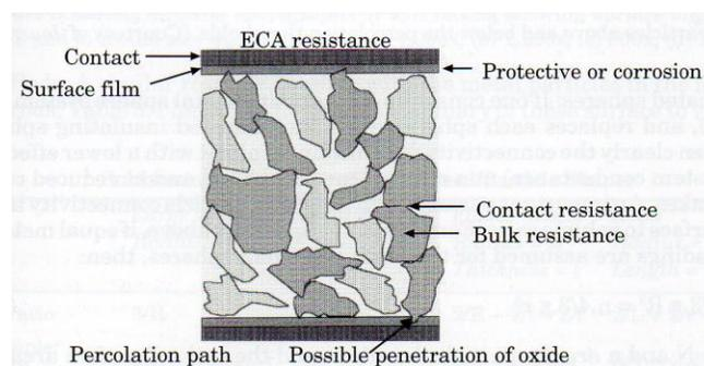
Figure 2 Electrical resistance elements in ICA [4].
