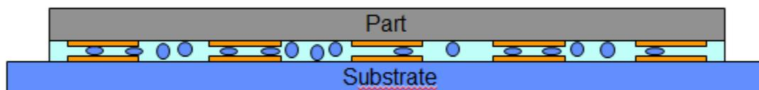
Figure 1 Schematic of ACA interconnection with deformable particles.
