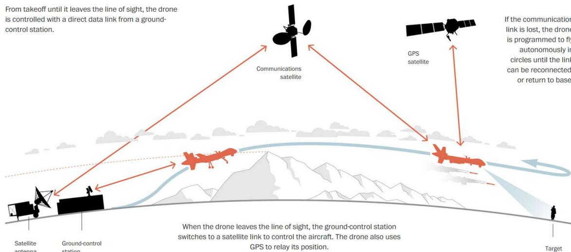
Figure 3: Typical Wireless Communication System for Military UAVs [4]
