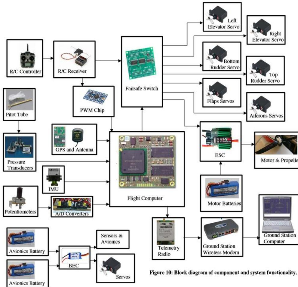
Figure 10: Block diagram of component and system functionality.
