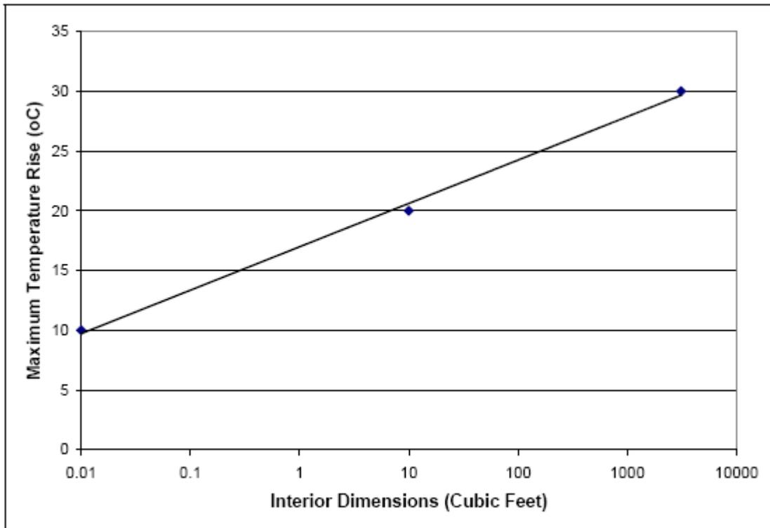
**Figure 4:** Maximum temperature rise at approximately 35C outdoor temperatures
