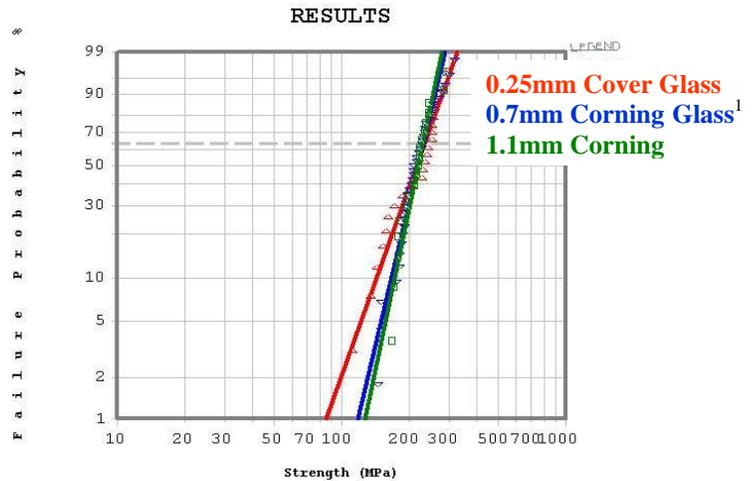
**Figure 2: Corning strength analysis – 'abraded' glass**
