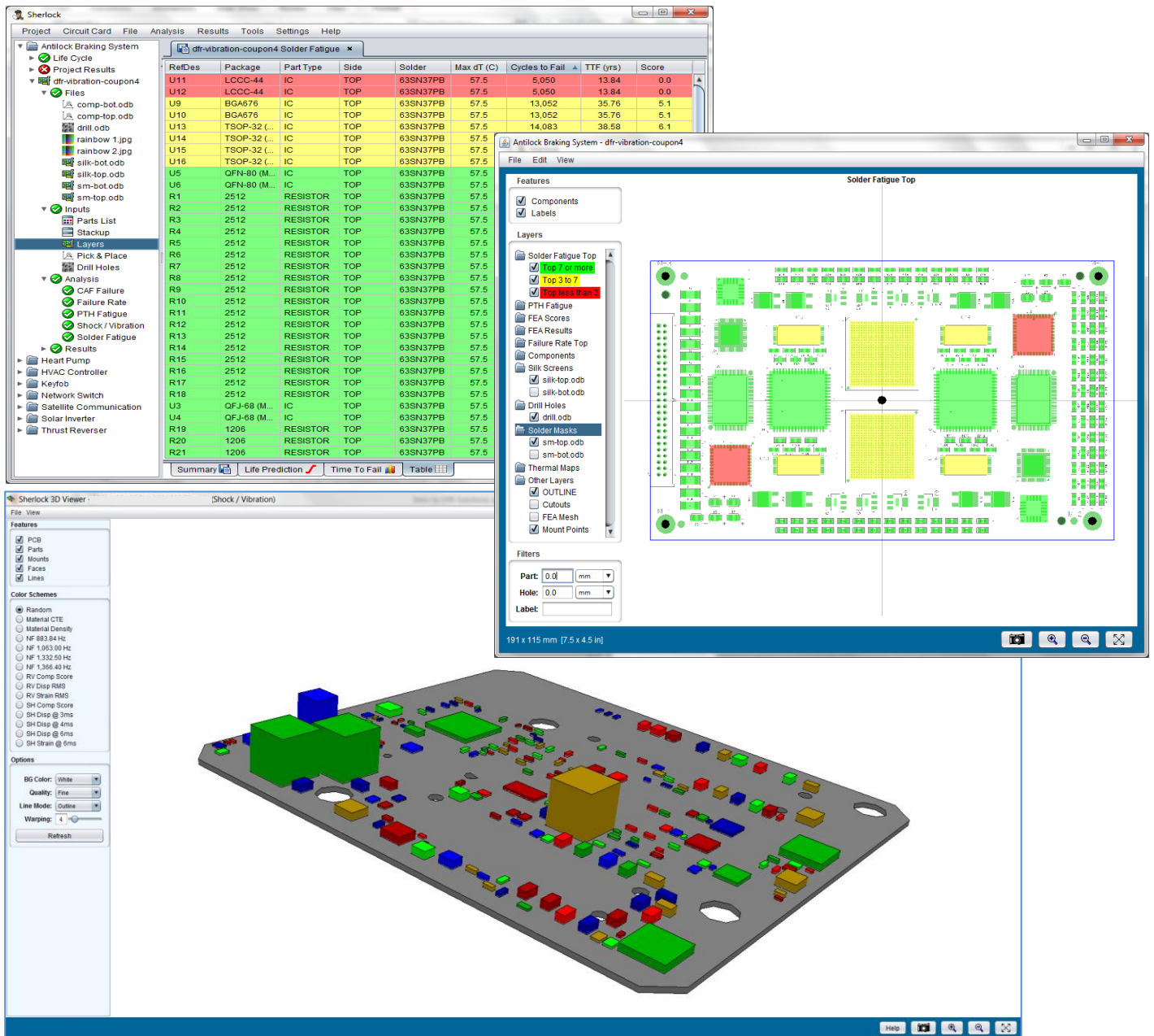
Figure 4: Pareto List and Color Coded 2D & 3D Graphic Representation of Component Failure Risks.
