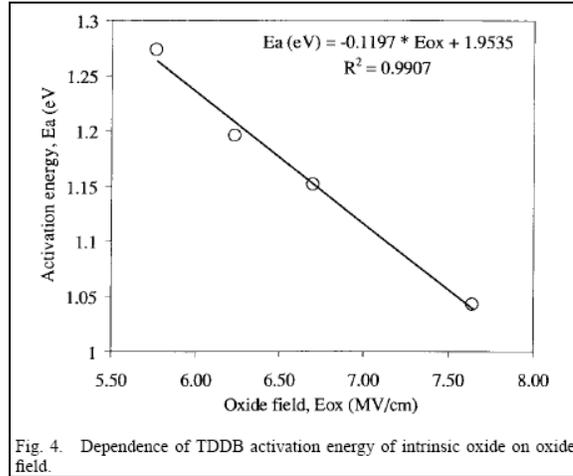
Fig. 4. Dependence of TDDB activation energy of intrinsic oxide on oxide field.
