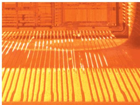
2. EOS-induced thermal overstress can even melt the wirebonds between a chip and its package.
