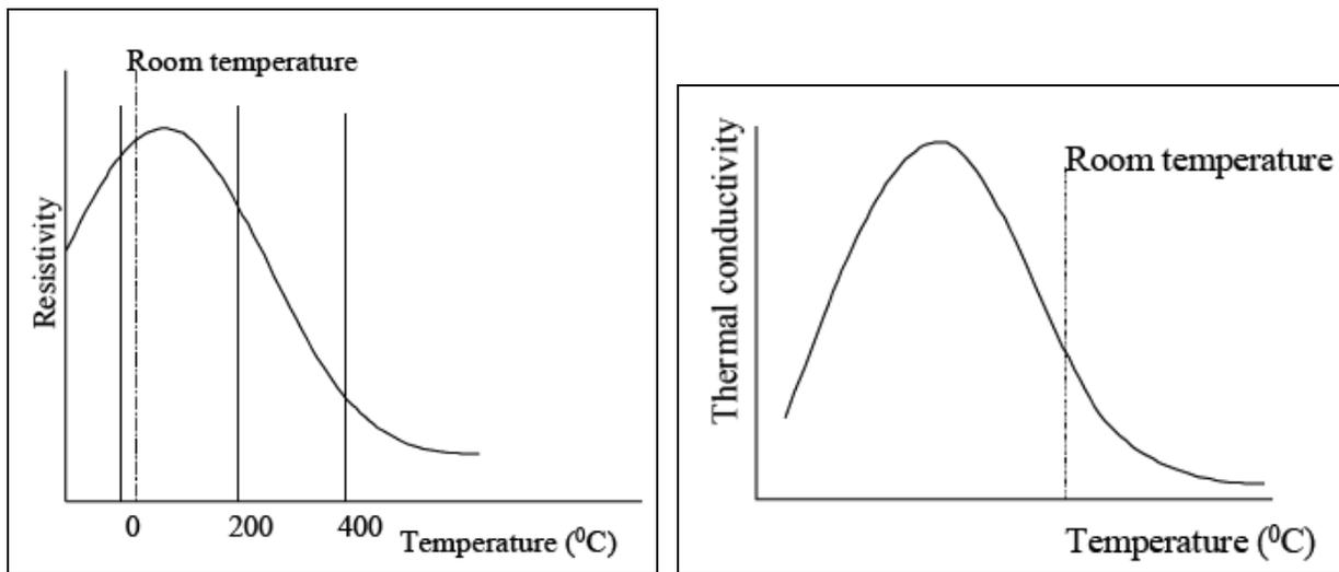
**Figure 5:** Change in resistivity and thermal conductivity of doped silicon as a function of temperature
