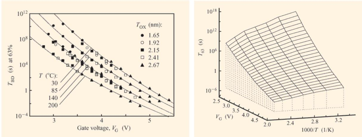
**Figure 3:** Time to breakdown as a function of voltage and temperature<sup>13</sup>
