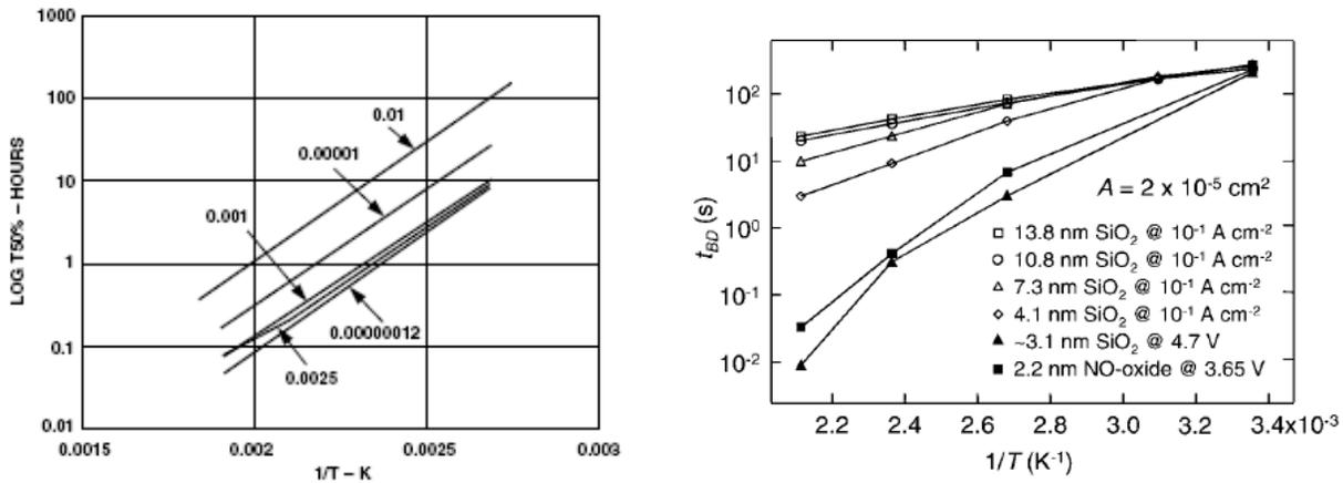
**Figure 4:** Thicker oxides displaying Arrhenius behavior (left), while thinner oxides display non-Arrhenius behavior (right)<sup>14,15</sup>
