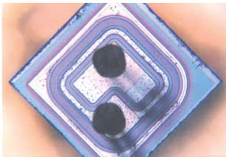
1. This bipolar junction transistor was damaged by thermal overstress caused by EOS. Note the hot spots in the base and emitter regions.
