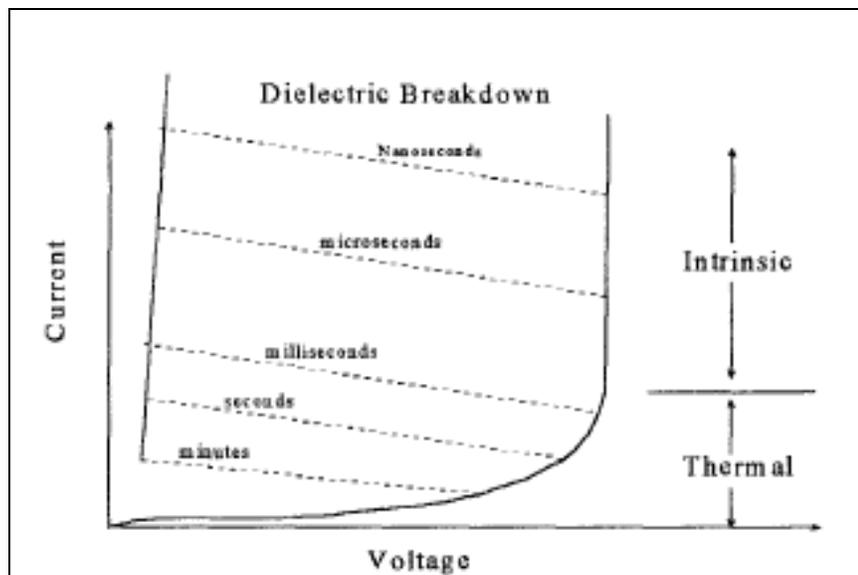
**Figure 2:** Transition between thermal and intrinsic breakdown in dielectrics<sup>12</sup>
