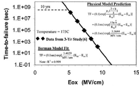
Fig. 10. Comparison of the Berman model and physical/thermochemical model when applied to longer-term/lower-field TDDB data. TDDB data collected for three years [6]. Data suggests that TF data can be extrapolated successfully from  $E_{bd}$  data. Here, breakdown was defined as the field at which failure occurs in 100 ms.
