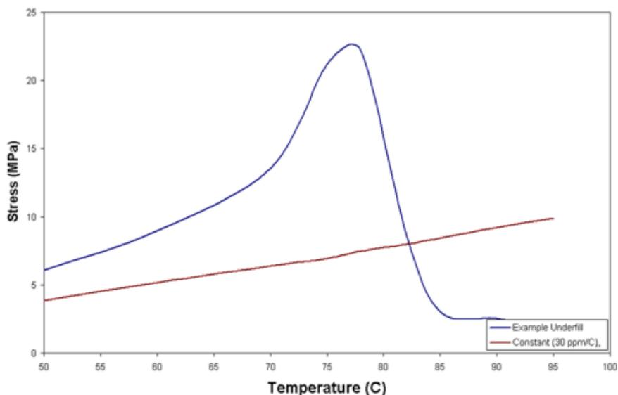
Figure 2. Tensile solder stress—elastic, compatibility of displacements.
