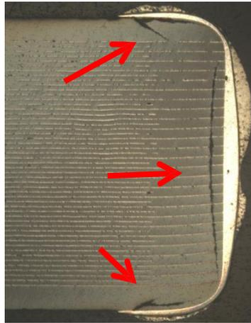
Figure 3 Ceramic Capacitor Thermal Shock Crack
