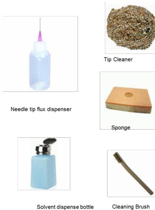
Figure 6 Manual Soldering Accessories
