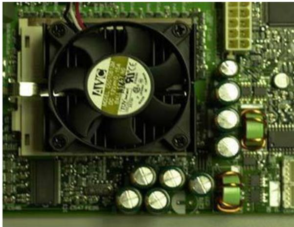
Figure 11 PTH Ecaps Close to Processor
