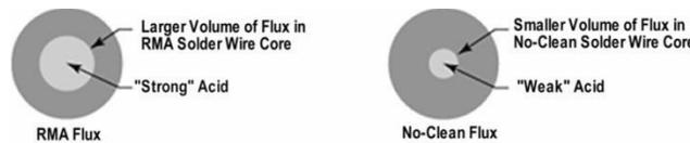
Figure 5 Flux Core Size vs Flux Type
