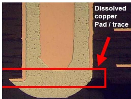
Figure 2 Cu Dissolution in a Solder Fountain
