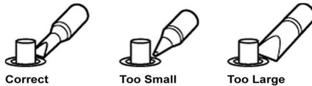
Figure 4 Solder Iron Tip Size Recommendations
