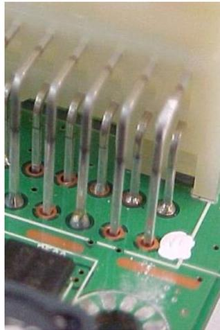
Figure 12 Insufficient PTH Hole Fill on Cu OSP
