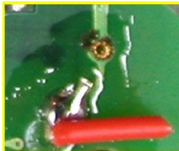
Figure 13 Excess Flux from Manual Soldering
