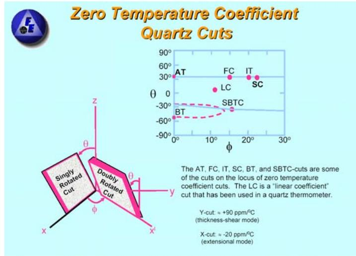
Figure 4: Crystal Cuts for Oscillators<sup>3</sup>
