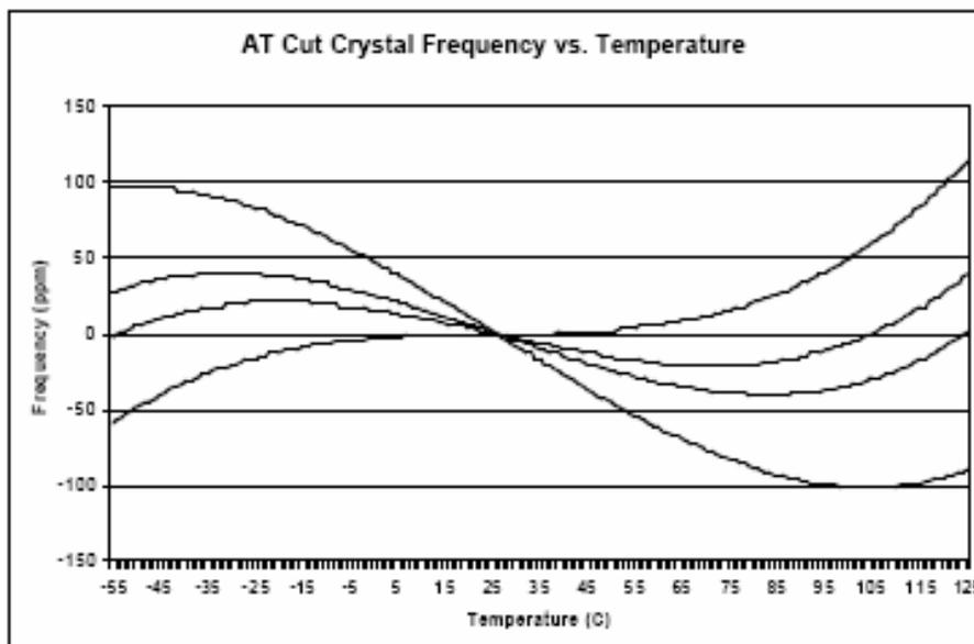
Figure 1: Frequency-temperature curves for the AT-cut crystal at different angle  $\phi$ <sup>1</sup>
