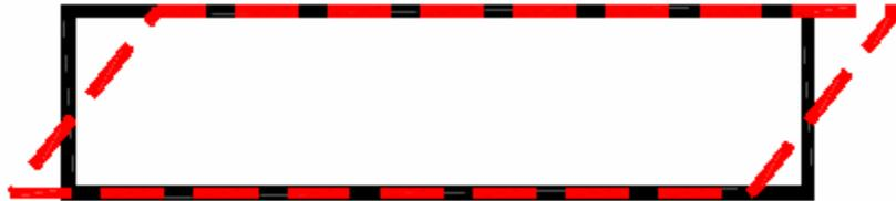
Figure 5: Thickness shear mode of vibration in AT or BT cut crystal<sup>4</sup>
