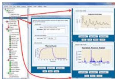
Figure 2. The user can define and save an unlimited number of test or field environmental and usage stress profiles to perform virtual test to field correlations and simulated aided testing studies.
