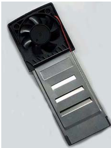
Figure 5: PCMCIA fan for supplemental cooling
