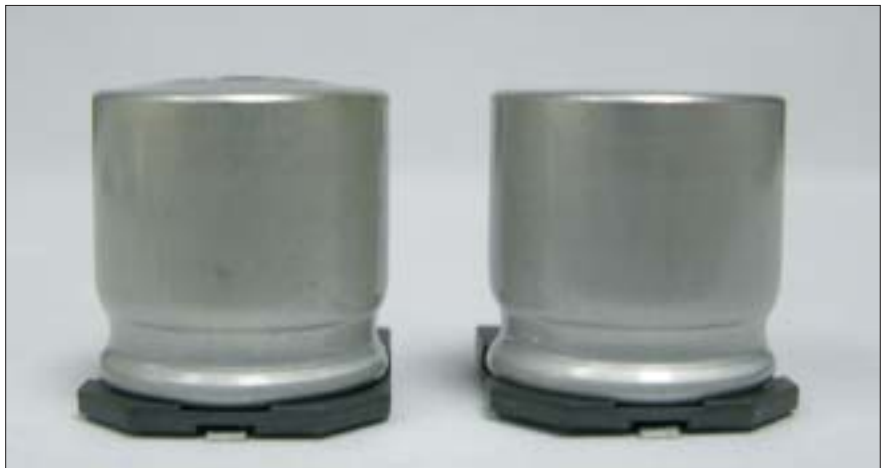
Figure 1: Aluminum Liquid Electrolytic Capacitor, on the Left, Has Experienced Case Distortion after an Extended Time at Pb-Free Reflow Temperatures
